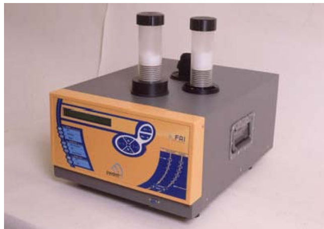
Figure 3.2 – Hydra (FAI – Instruments) sampling unity.
