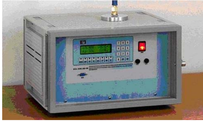
Figure 3.13 – OH-610-C impactor measuring and control unit integrated with pump and motor, connection cables and electric fittings.
