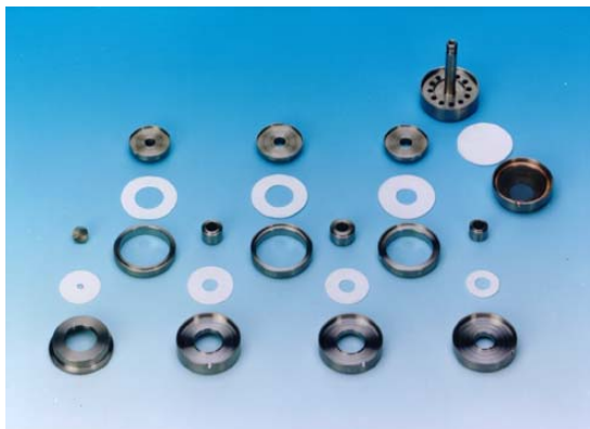
Figure 3.11 – The cascade impactor OH-610-C (Kálmán System) in a disassembled state. In each stage the collection surface is a quartz filter substrate.
