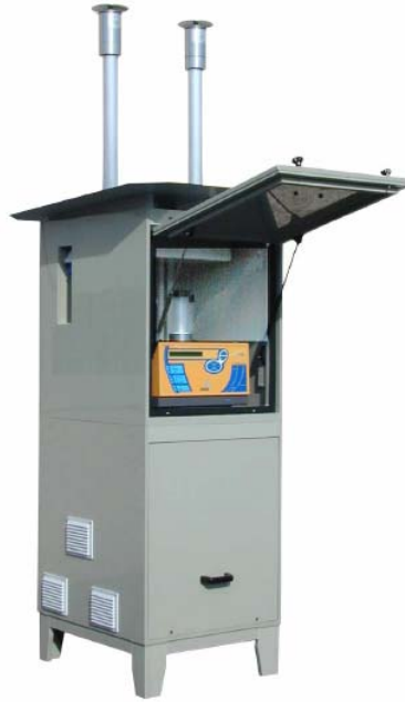
Figure 3.1 – Hydra dual sampler (FAI-Instruments).
