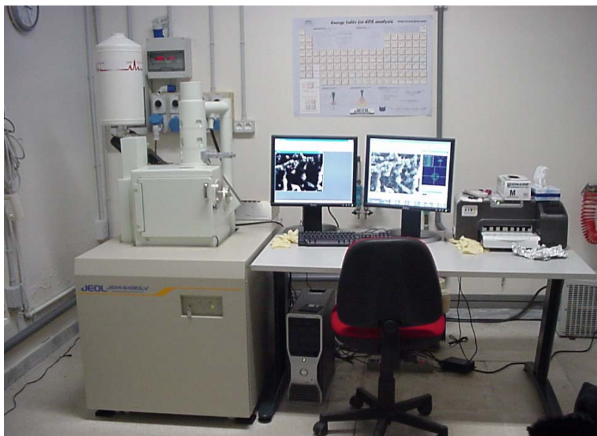
Figure 4.11 – The scanning electron microscope (JEOL, model JSM-6480LV), equipped with an energy dispersive X-ray (EDX) system (model EDS 2000) of Physics Department of University of Salento.
