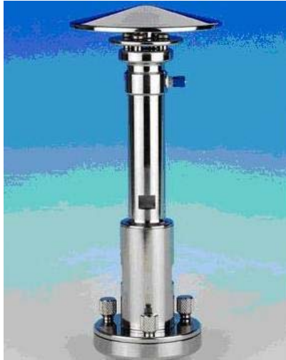
Figure 3.9 - The 7-stage cascade impactor OH - 610 - C - Kálmán System.
