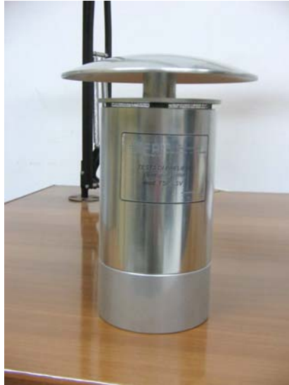
Figure 3.4 – LSV sampling inlet (2.3 m 3 /h) of Hydra dual sampler.
