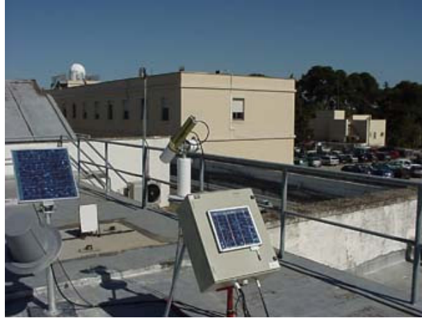
Figure 1.2. Picture of the sun photometer located on the roof of the Physics Department of Salento's University.
