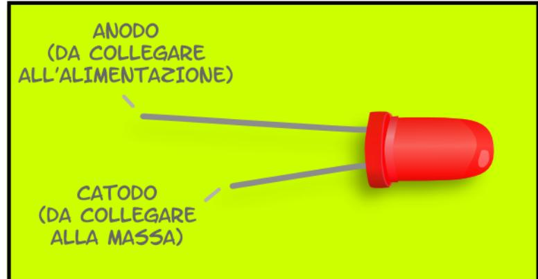
QUANDO LA CORRENTE CIRCOLA NELLA DIREZIONE GIUSTA UN **LED (DIODO AD EMISSIONE LUMINOSA)** SI ACCENDE. COLLEGHIAMO UN LED ALLA BREADBOARD E PROVIAMO A CONTROLLARLO SCRIVENDO DEL CODICE, CIOE' CON UN PROGRAMMA.
