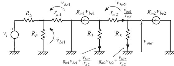
$$v_{out} = R_5 \left( v_{be2} g_{m2} + \frac{v_{be2}}{r_{\pi 2}} \right),$$
