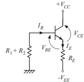
$$V_{EE} - V_{BE} = (R_1 + R_2)I_B + R_E I_E = I_E \frac{R_1 + R_2}{\beta + 1} + I_E R_E,$$
