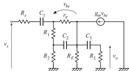
$$R_p \equiv \frac{1}{\frac{1}{R_2} + \frac{1}{R_E} + \frac{1}{R_L}} \approx 107.23 \text{ k}\Omega.$$
