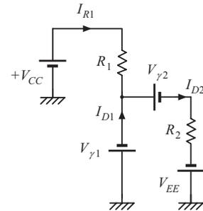
$$I_{R1} = \frac{V_{CC} + V_{\gamma 1}}{R_1} \approx 1.07 \text{ mA},$$
