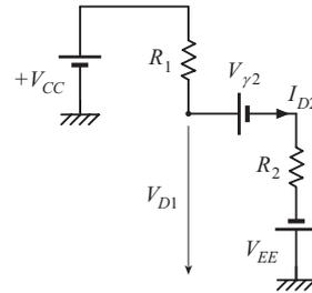
$$V_{CC} + V_{EE} - V_{\gamma 2} = (R_1 + R_2)I_{DL},$$
