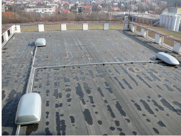
Figure 3.3: Picture of a ALTA station in Canada, the boxes contain the scintillation detectors.
