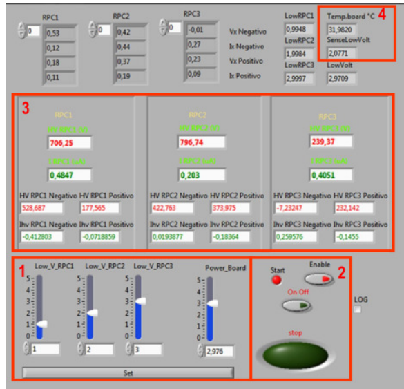
Figure 3.19: LV/HV control system graphic interface. 1. LV to DC/DC converters; 2. the module's status; 3. HV and currents from MRPCs; 4 Temperature of the NI board and voltage from FE boards.
