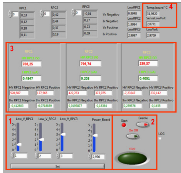
Figure A.4: LV/HV control system graphic interface. 1. LV to DC/DC converters; 2. VCS status; 3. HV and currents from MRPCs; 4 Temperature of the VCS board and sense voltage from FE boards
